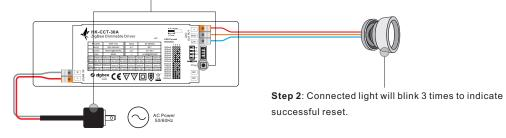
Note: 1) If the device is already at factory default setting, there is no indication when factory reset again . 2) All configuration parameters will be reset after the device is reset or removed from the network.
